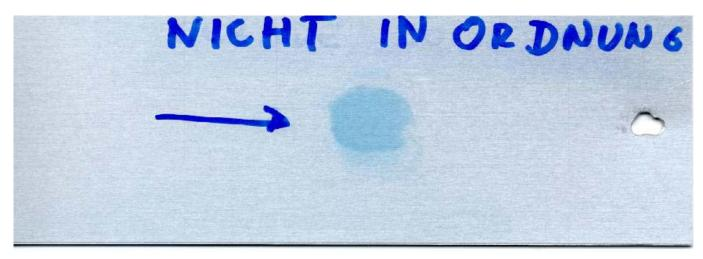
As a reference for the "open porosity" of the oxide layer a specimen could be used treated with one drop of an acid solution and properly rinsed with demineralised water prior to applying the test solution.
